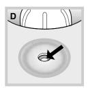
9. Take it out of the refrigerator and turn the knob clockwise to the CLOSE position to avoid accidental opening (see figure A). The absence of air inside the container is indicated by the valve at the bottom (see figure D).
